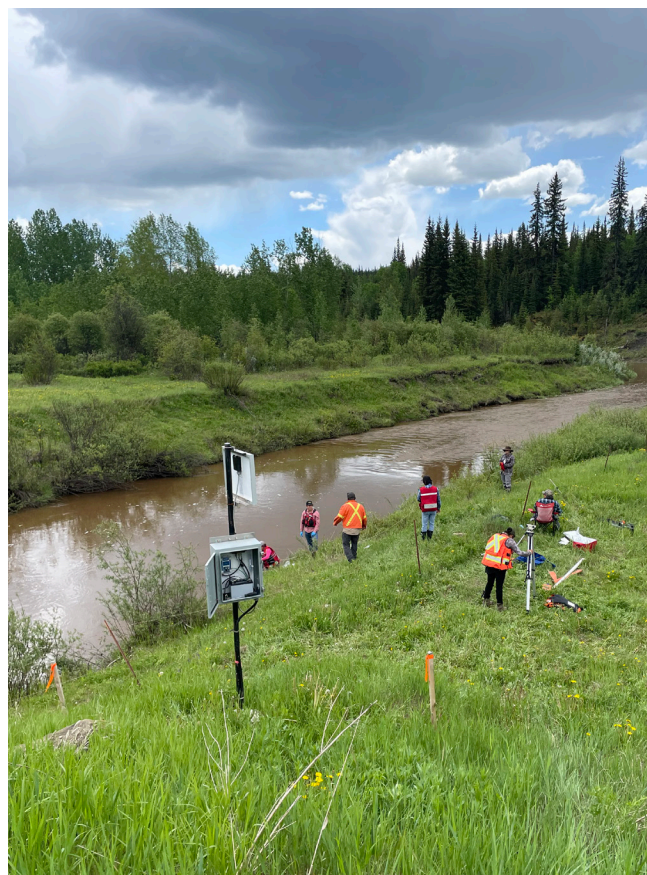
High flow measurement and water level surveying on Blueberry River.
