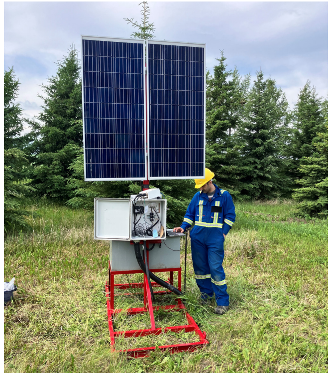
Redeployment of seismic monitoring station MONT1 in Parkland, B.C.
